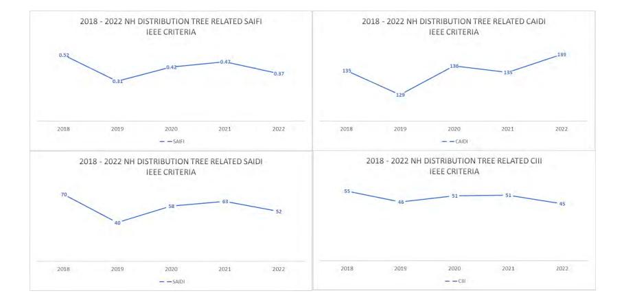
Section 1.4 SAIFI, SAIDI, CAIDI, CIII – Distribution (excluding Substation) Equipment Failures – IEEE Criteria
